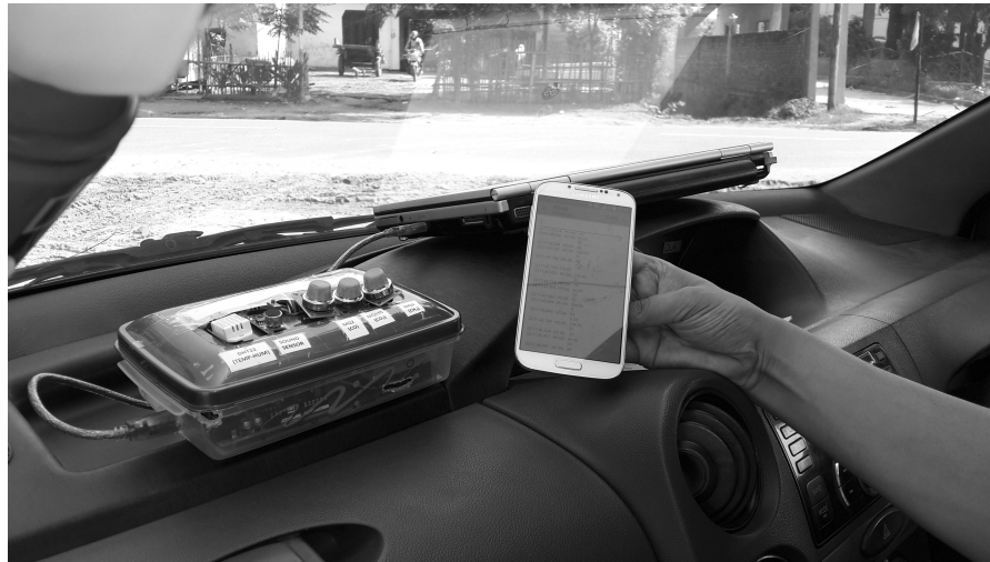
Fig.2: Data collection setup: The IoT sensing system placed inside a vehicle to collect air quality data
