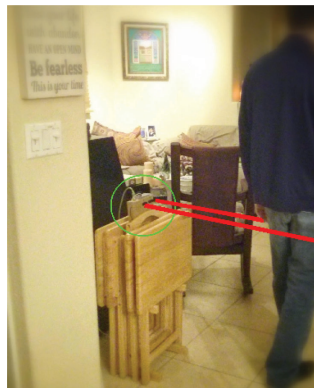
An experiment where a resident is crossing in front of a node is shown. Drawn red lines represent the beams emitted by the IR distance sensors. The placement of the node is indicated with a green circle.
