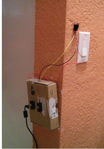
Placement of a node at a crossing of two regions. The light sensor is placed outside, pointing towards the light source of the region.
