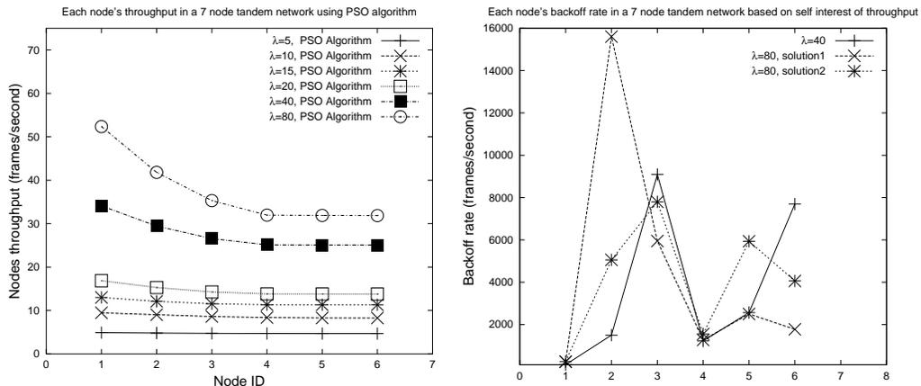
(a) Each node's throughput in a 7-node tandem network using a PSO algorithm. (b) Each node's backoff rate in a 7-node tandem network using a PSO algorithm.
