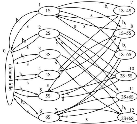
Channel Utilization Model in a 7-node tandem network
