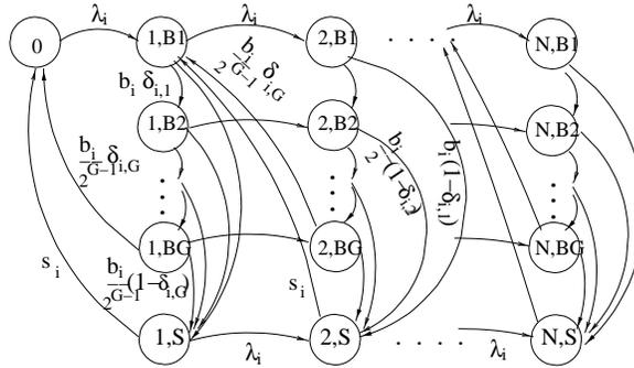
(b) Single node markov chain with the multi-stage back off process.
