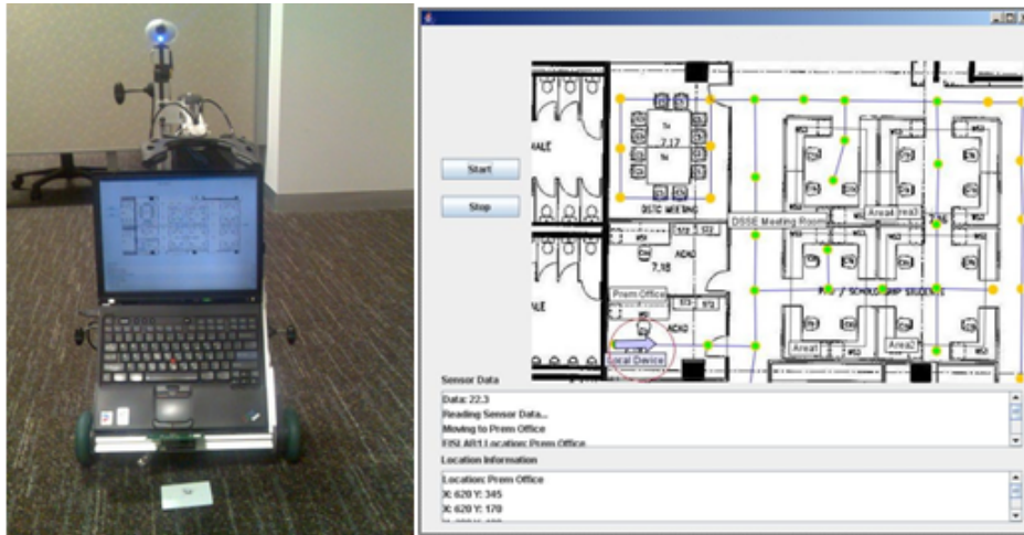
Figure. 7: The Data Mule Framework implemented on a mobile robot platform and Screenshot of the Data Collection interface running on the Data Mule
