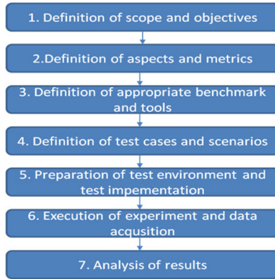
Figure 3: Steps of the load testing procedure
